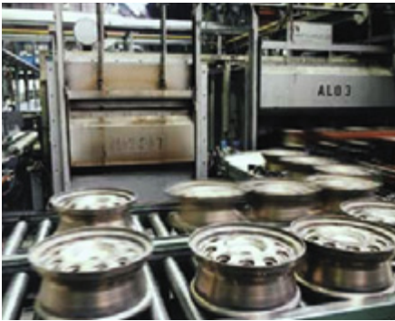
Aluminium industry: curing oven for wheel rims
